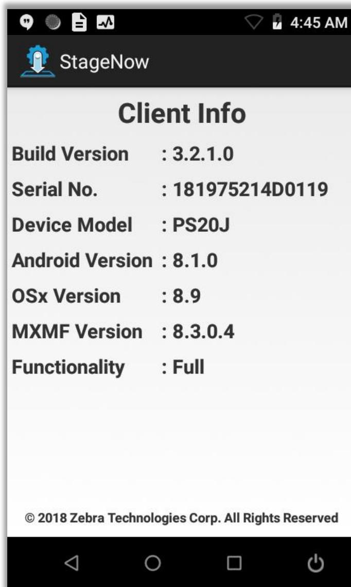
This StageNow version is 3.2.1.0 (minimal version should be 3.2) and MX version is 8.3.0.4 (minimal version should be 8.3).
